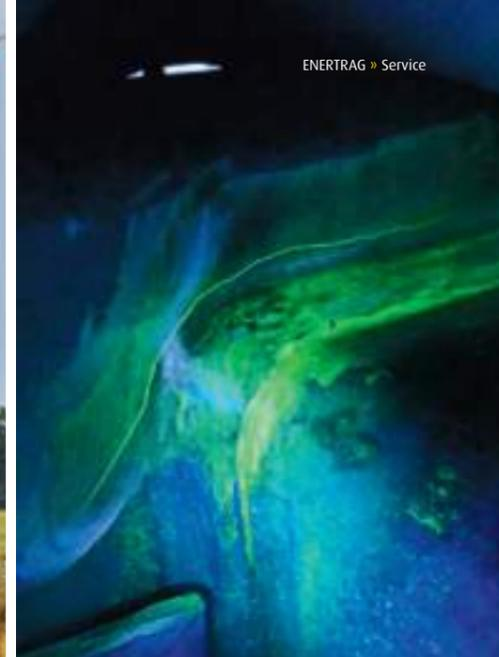
**Forgoing inspections can be disastrous:** it takes a non-destructive inspection to reveal a minute crack in the generator frame. Fluorescent magnetic particle powder and UV lamps do the job.
