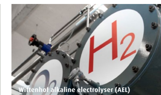
Wittenhof alkaline electrolyser (AEL)
